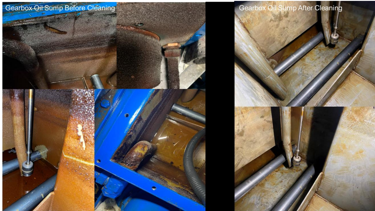
T1 – Oil Soluble cleaner to remove/ soften deposits followed by manual clean
