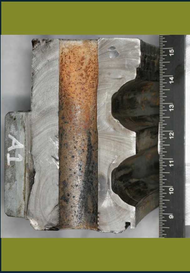
Photograph of a race from a failed blade pitch bearing, sectioned through a bolt hole; "beach marks" typical of fatigue crack growth are evident
