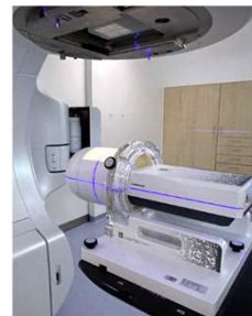
Figure 4: MyQA SRS setup in room under gantry head. MyQASRS device fits inside cylindrical phantom for measurements.
