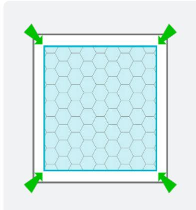
Figure 1: Illustration of surface shrinkage upon wetting test
