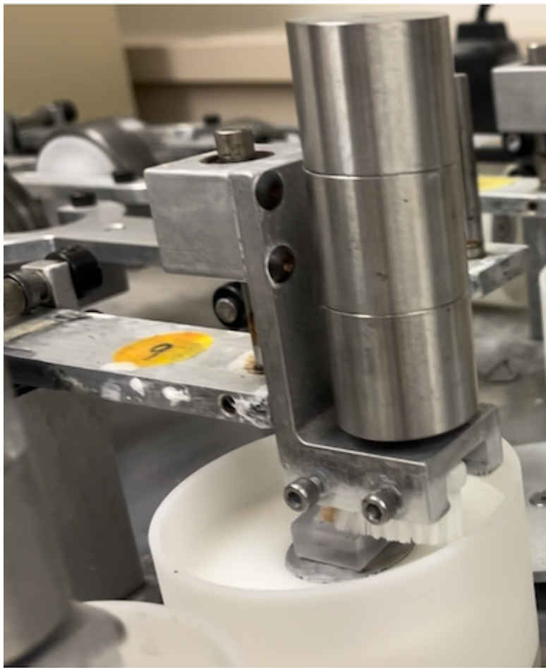
Mounted weighted sample, simulating brushing force, with toothbrush attached, and intact molar.
