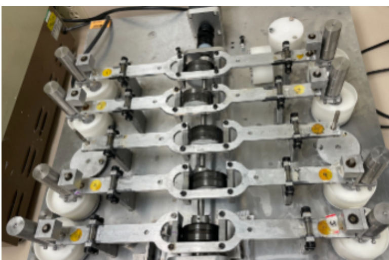
Tooth brushing machine with the brush attachments moving back and forth, and the sample cups (occlusal surface) rotate
