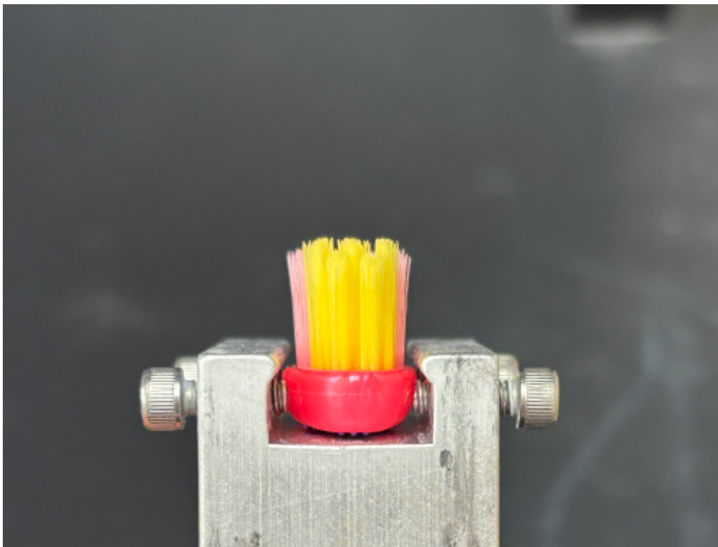
Tooth brush placement in holder for toothbrushing machine prior to simulated brushing cycles.
