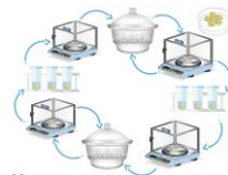
Figure 3. Cycle of Water Sorption and Solubility Testing. Stable mass (M1), Mass after water exposure (M2). Final weighing with stable mass (M3). WS = (m_2 - m_3)/V ; SL = (m_1 - m_3)/V
