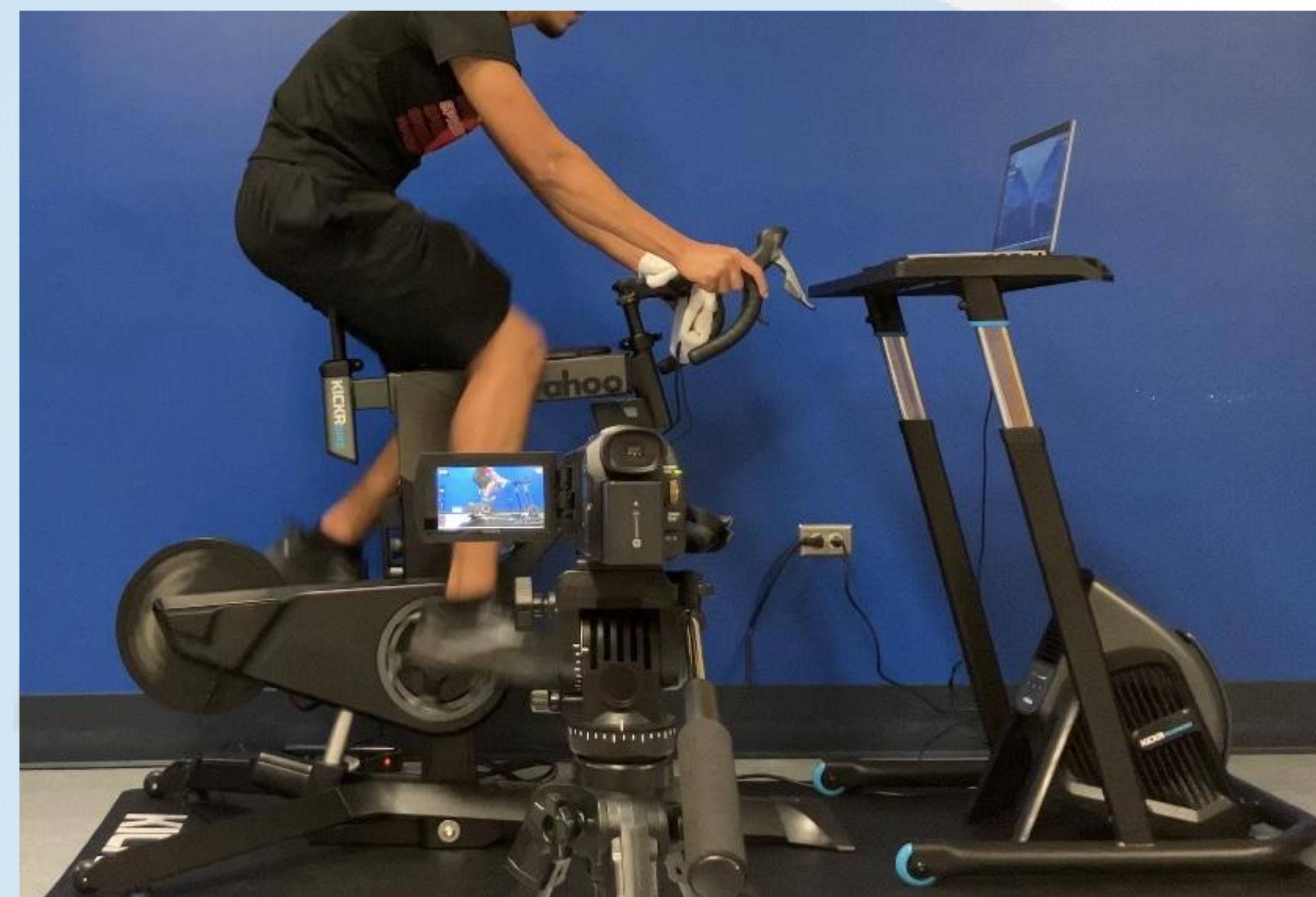
Figure 1. Data collection setup showcasing the Wahoo KICKR BIKE, video camera, and laptop for AR cycling software and kinematic analysis.
