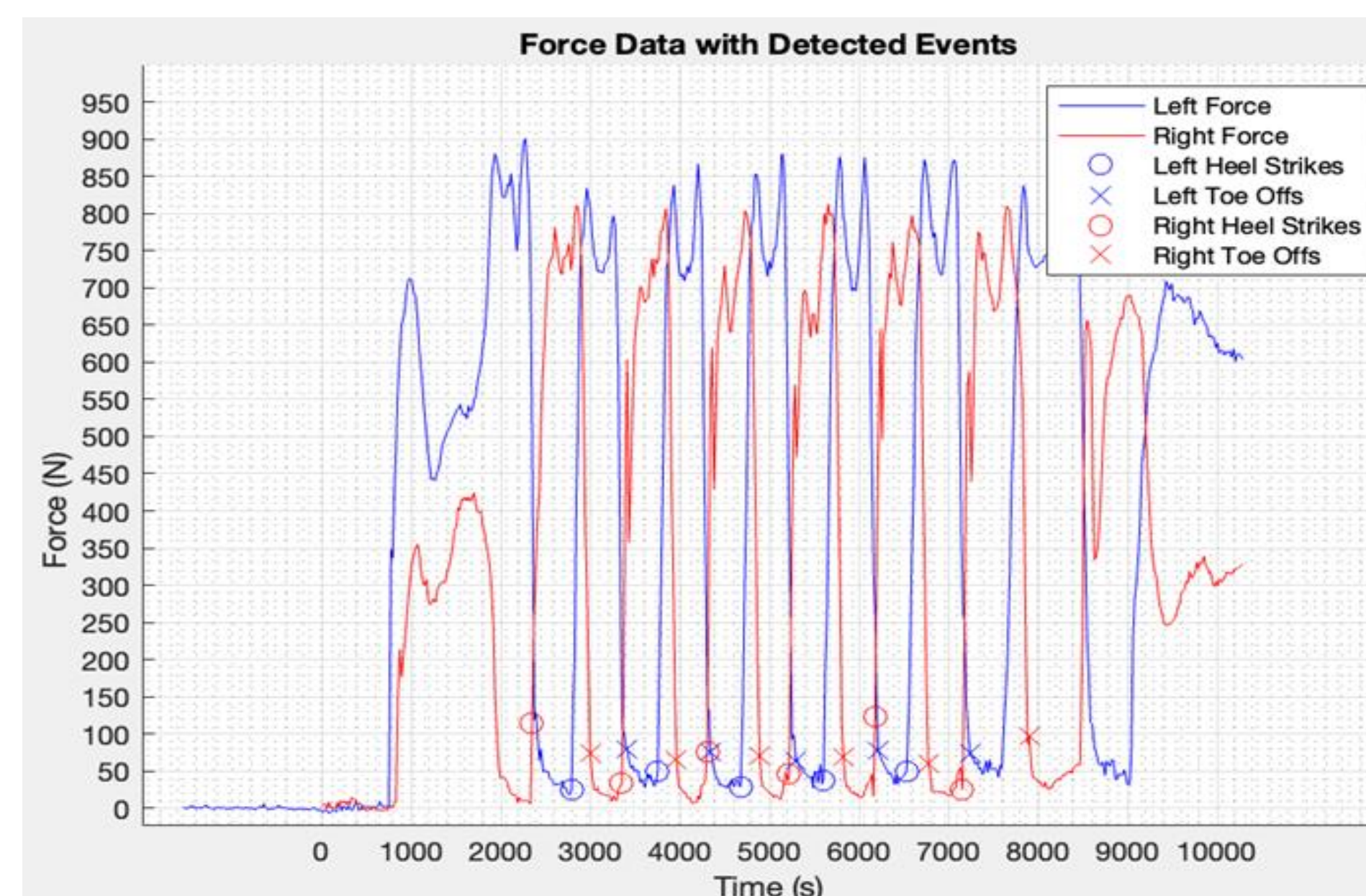
Figure 1: A representative Force vs Time chart for a single gait analysis trial
