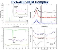
XRD shows reduced amorphous nature and GEM peaks (27-75°); ASP peaks absent after washing. Peak shifts indicate polymorphic transitions. DSC: new peak at 154.5 °C and broad peak at 238.1 °C confirm enhanced thermal stability. Results align with TGA
