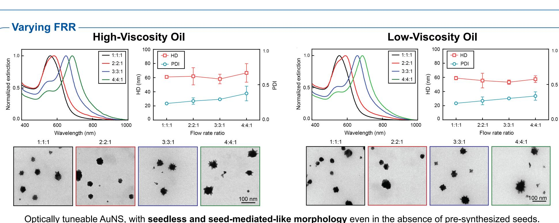
Higher fraction of seed-mediated-like AuNS was obtained with lower viscosity oil at low and moderate FRR.
