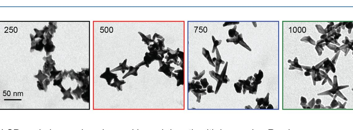
Optically tuneable AuNS with seedless morphology, red shifting LSP peak, increasing size and branch length with increasing R value.
