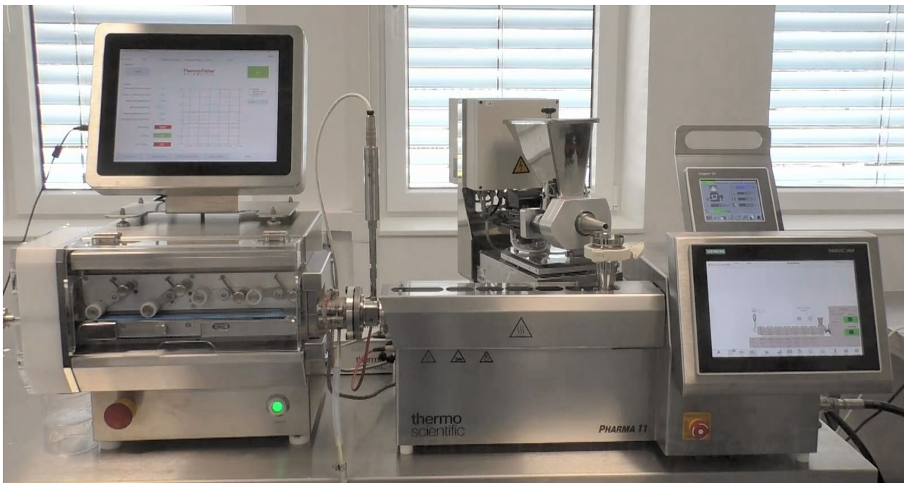
Figure 1. Extrusion setup for hollow tube extrusion with Pharma 11 twin-screw extruder, gravimetric RotoTube feeder, Pharma 11 catheter die, and pulling and cutting to the required length and diameter control via the CaliCut post-extrusion system.
