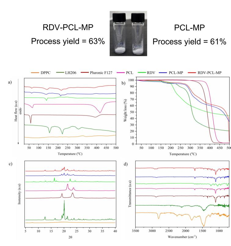
a) DSC, b) TG, c) DRX, and d) FTIR, illustrating the thermal transitions, stability, crystallinity and molecular interaction of excipients: DPPC, LH206, Pluronic F127, RDV and formulations containing or not RDV: PCL-MP and RDV-PCL.
