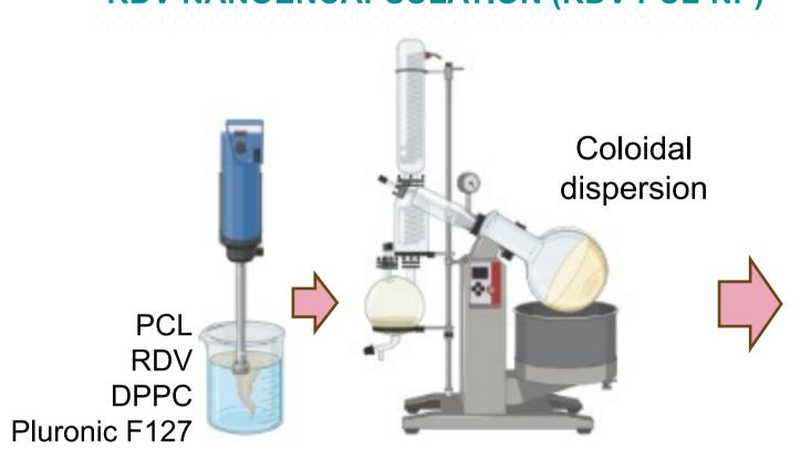
NPs of PCL were produced by emulsiondiffusion-solvent evaporation and characterized by DLS and zeta potential DPPC was incorporated to facilitate pulmonary delivery.
