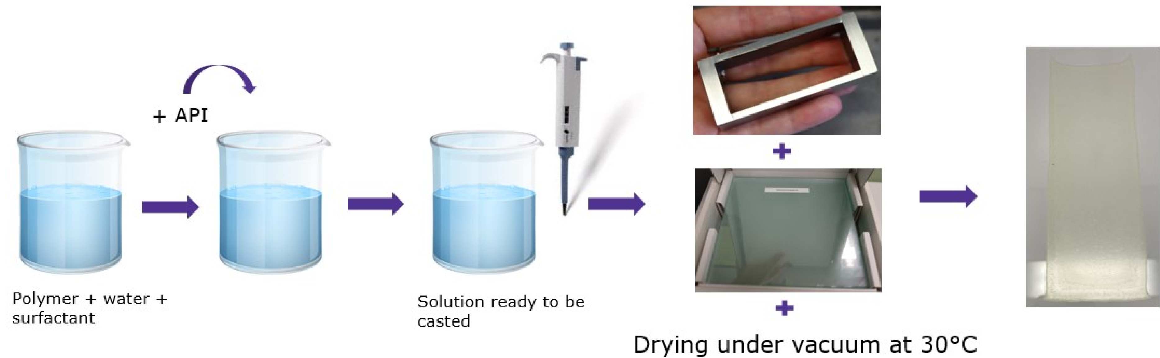
Figure 1: overview of manufacturing process of PVA orodispersible films.
