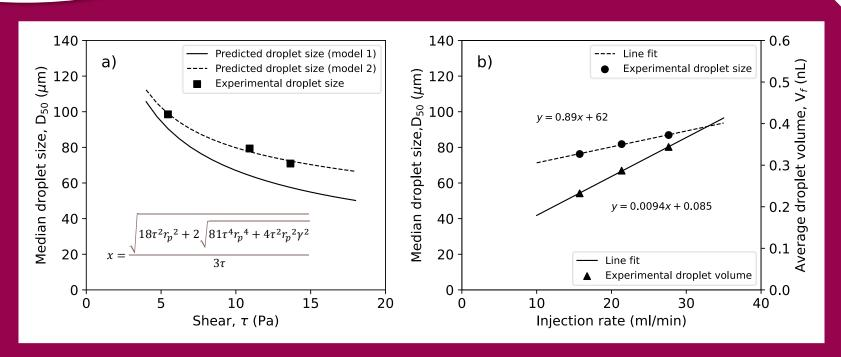
(a) Median droplet diameter  $D_{50}$  as a function of the shear  $\tau$  at a dispersed phase flowrate of 16 ml/min and the predicted droplet diameter from the force balance model.
