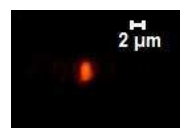
Figure 7: The transmitted signal of a HeNe-laser source inside a silicone waveguide, detected by a CCD-camera
