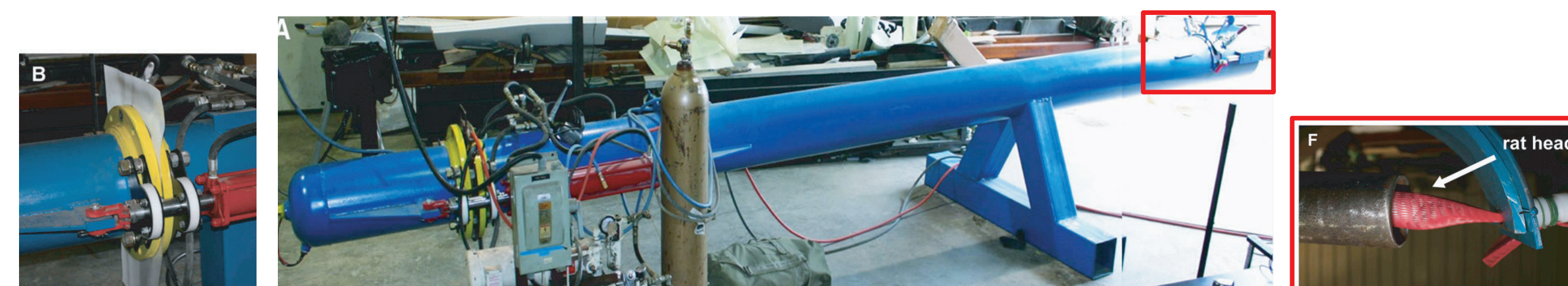
Figure 4. Blast device showing perforatable (B) membrane and animal location (F). Modified from Reneer et al., Journal of Neurotrauma, 2011.
