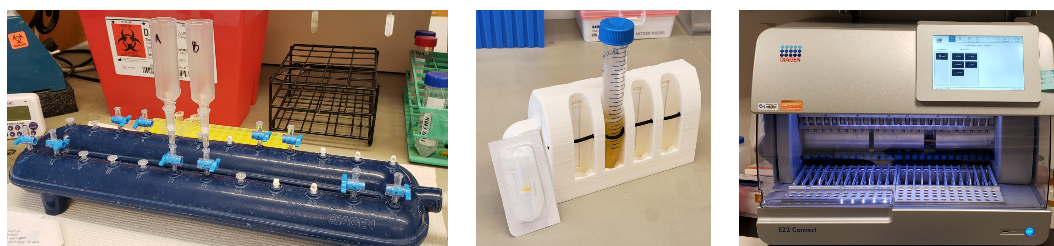
Figure 1. Methods Used by QIAGEN cfDNA Extraction Kits. Left image: Vacuum and columns used for the Circulating NA kit. Middle image: Magnet and spin column used for the MinElute kit. Right image: EZ2 instrument used for the automated EZ1&2 kit.
