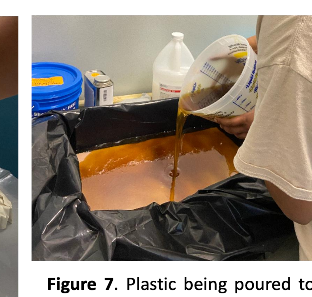
Figure 7: Plastic being poured to make permanent plastic mold for the chest wall of economy model.
